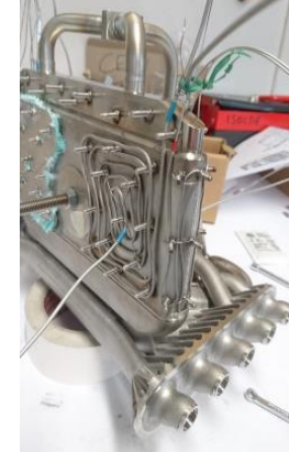
LIEBE ion source sub assembly with heating elements
