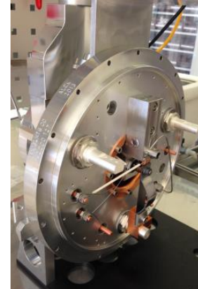
LIEBE ion source sub assembly with heating elements
