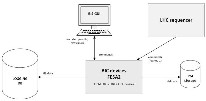
(not a magnet protection system per se, provided here as an example of a lower complexity system following a very similar architecture)
