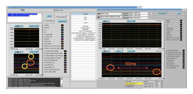
Due to differences in timestamping source and mechanisms (local vs remote/gateway timestamping, central timing vs NTP...), identical signals can get timestamped with insufficient accuracy
