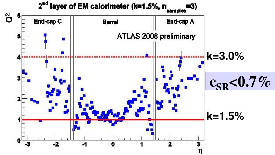
→ Signal reconstruction under control on the whole calorimeter coverage
