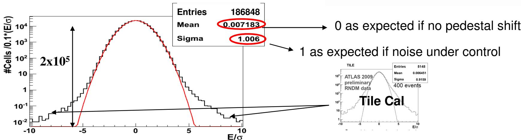
→ Calorimeter cells under control
