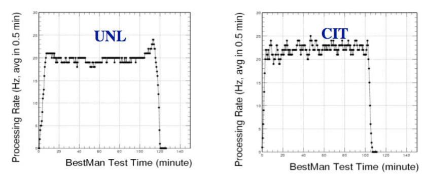
The effective processing rates of UNL, CIT and UCSD are essentially the same. Average at 20 Hz, peak at ~25 Hz. It also shows the latency in running the command doesn't affect the scalability of the BeStMan.
