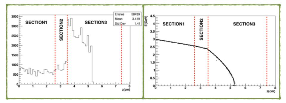
Carbon interaction vertices Final kinetic energy of the position along the axis carbon ions inside ECC as function of the depth.
