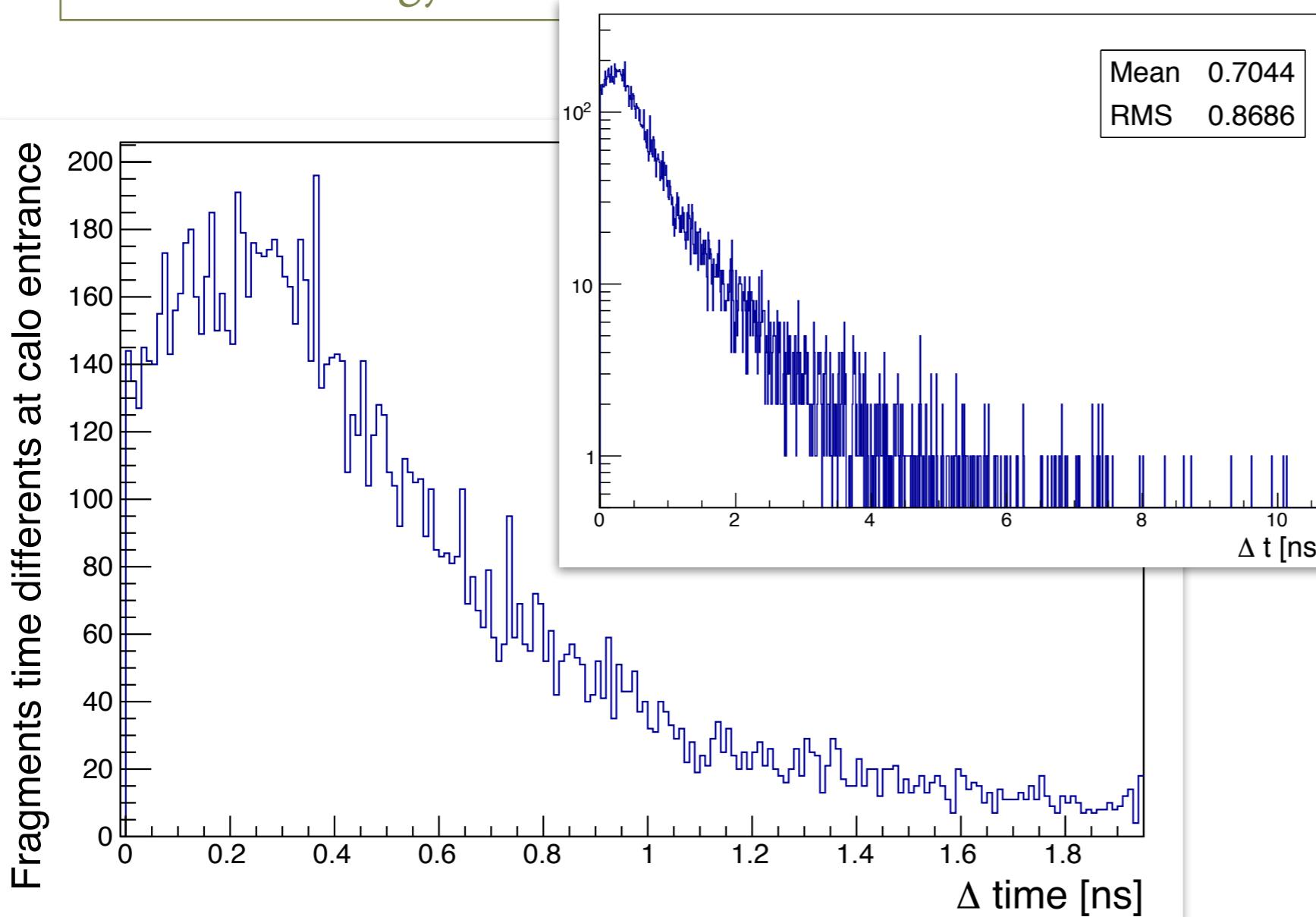
Most of the events occurs in few ns.. if the timing of the events is an stringent requirement the time-resolution of the calorimeter becomes a stringent parameter.
