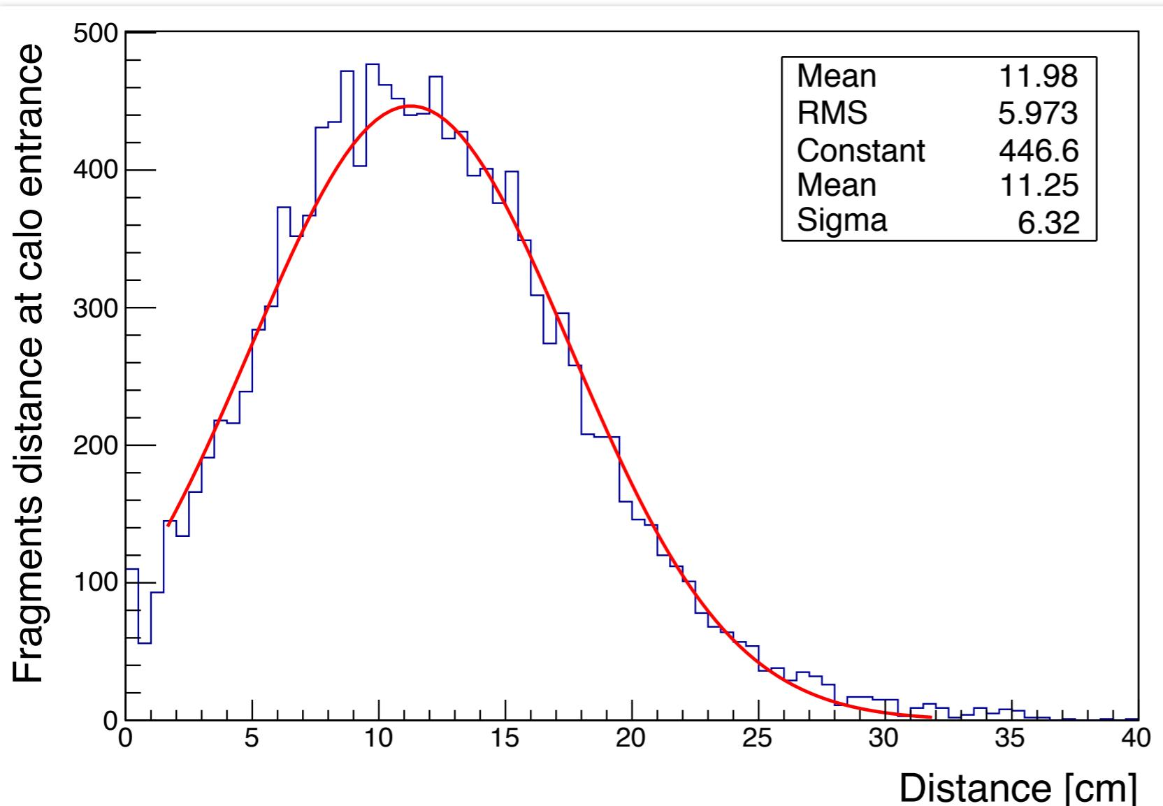
The size of a single BGO crystal is 2 cm, therefore we can assume that only a **very small fraction** of events will present multiple-fragments impinging on **two adjacent crystals**.
