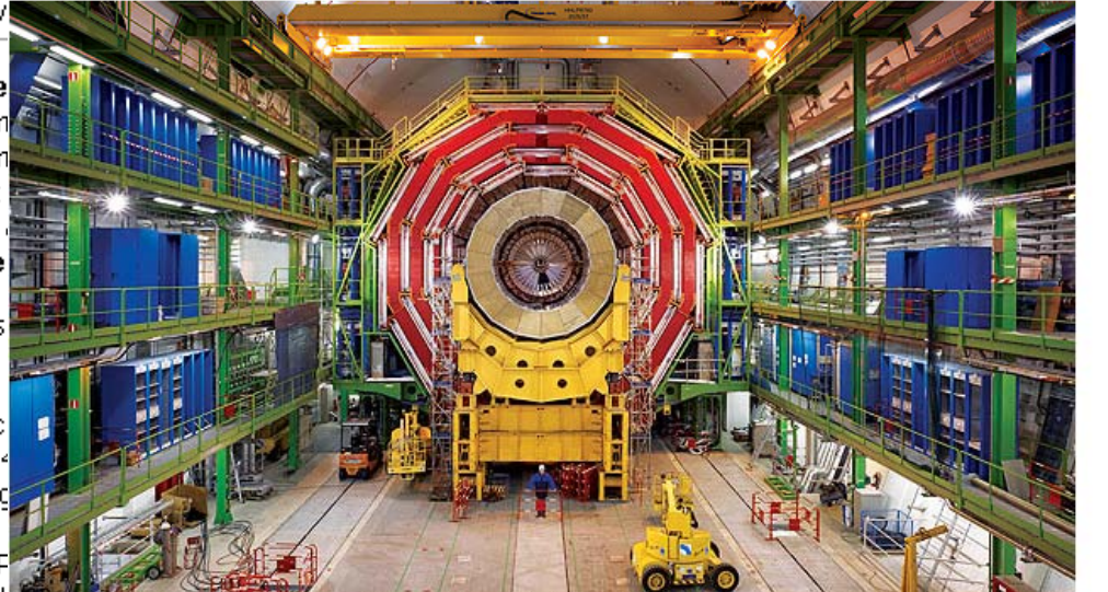
Various magnets of the paradoxically named Compact Muon Solenoid experiment are moved into position at the Large Hadron Collider facility deep under the French-Swiss border.
