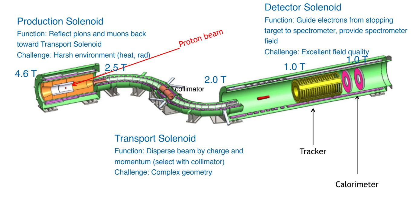
The overall grade of the field increases muons on target and electrons in spectrometer, as well as preventing particle traps
