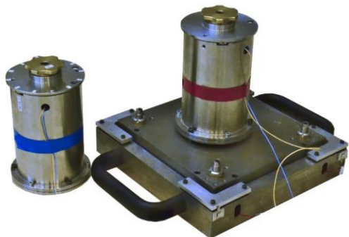
- LAPP active foot + LAPP sensors (one on ground used to monitor ground motion and 1 on top used in feedback)
