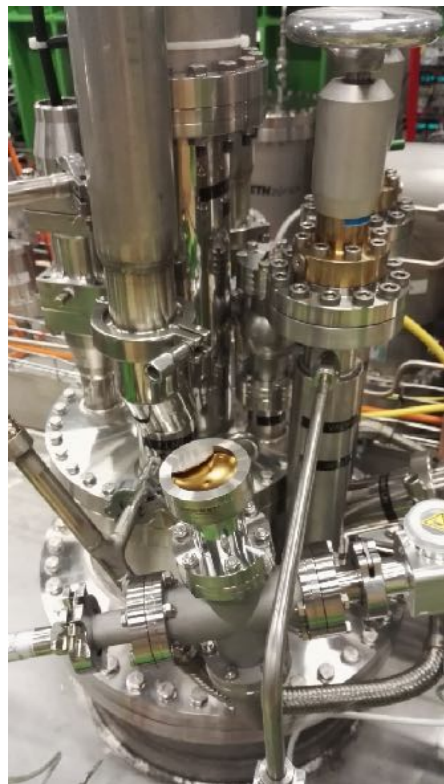
some leaks on pump tower flanges
