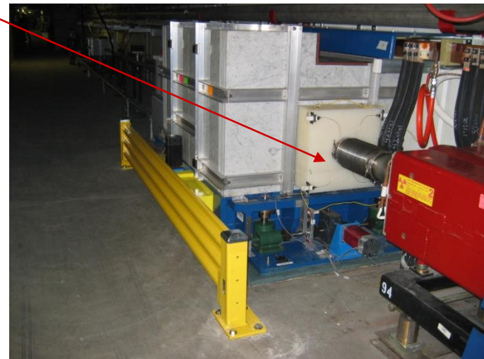
Marble shells of a brand-new collimation system at Fermilab MI
