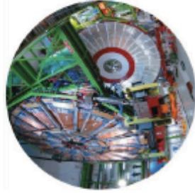
Part of the Compact Muon Solenoid particle detector is lowered into place several hundred feet below ground. COURTESY CERN
