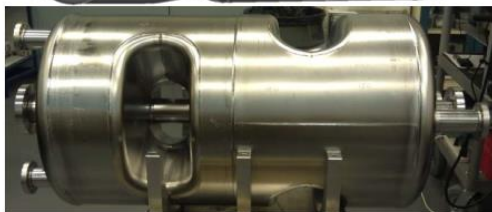
500 MHz, \beta_0 = 1 Double-Spoke Cavity
