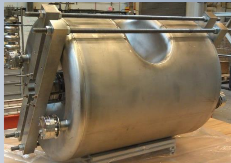
325 MHz \beta=0.82 Single Spoke Cavity
