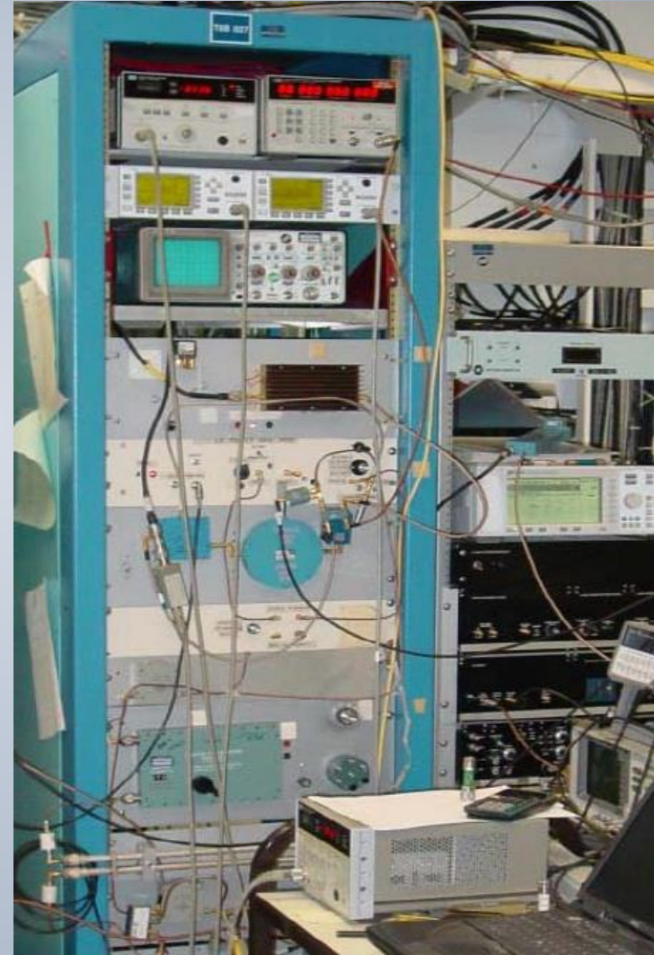
JLAB 0.5-3GHz VCO PLL system for R&D
