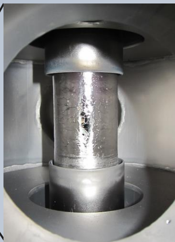
Nb cathode with permanent magnets inside and Nb anodes
