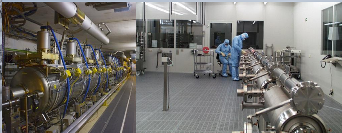
LHC cryomodule couplers above the cavities
