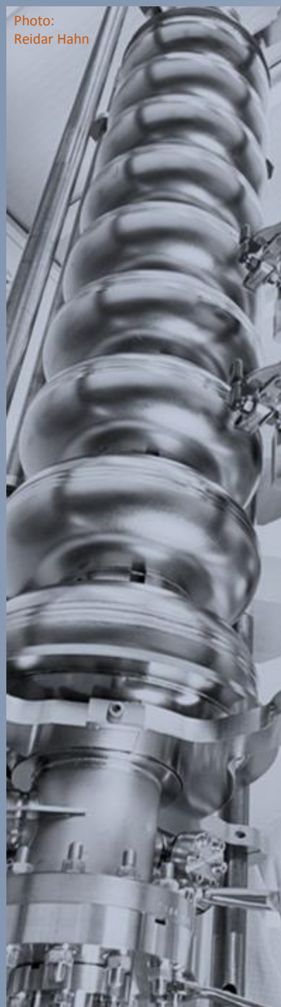
LHC cryomodule couplers above the cavities
