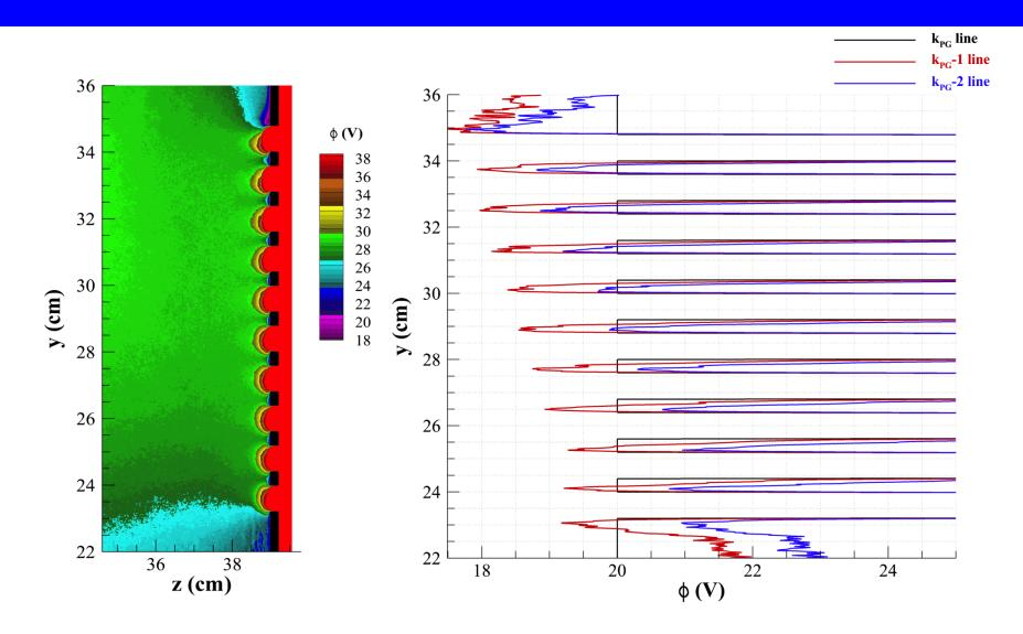
All the quantities show a marked top-bottom asymmetry due to the aforementioned magnetic drifts. Meniscus shape and potential well are not uniform along the different apertures.
