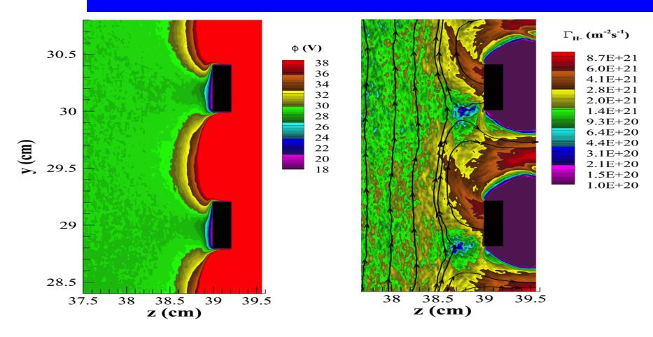
The meniscus shape is presented as asymmetrical lobes with a penetration length inside the source increasing from the bottom to the top aperture. Even the potential well attached to the PG surface is not uniform between two adjacent apertures, but it reaches a maximum depth of 2 eV from one side, the upper one, of the aperture and it is absent on the other side, the lower one.
