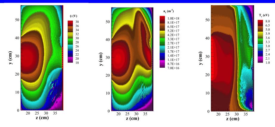
This clearly shows the working principle of magnetic filter field: making the electron transit time larger and the flux almost entirely parallel to the magnetic field lines in the filter region, electrons reduce their energy by collisional events and move faster along transversal direction. These effects reduce both the electron temperature and density downstream of the magnetic filter region.
