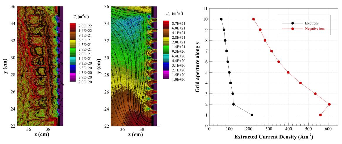
Due to the inhomogeneous plasma condition induced by the magnetic filter field, the extracted currents show a non uniform distribution along the different apertures.
