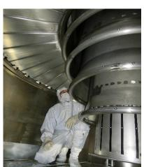
1MV was sustained stably and repeatedly during three days test period.
