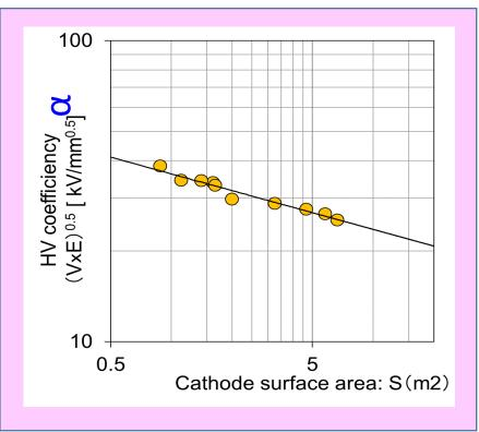
Experimental scaling to design large accelerator with large grid and large support system is established.
