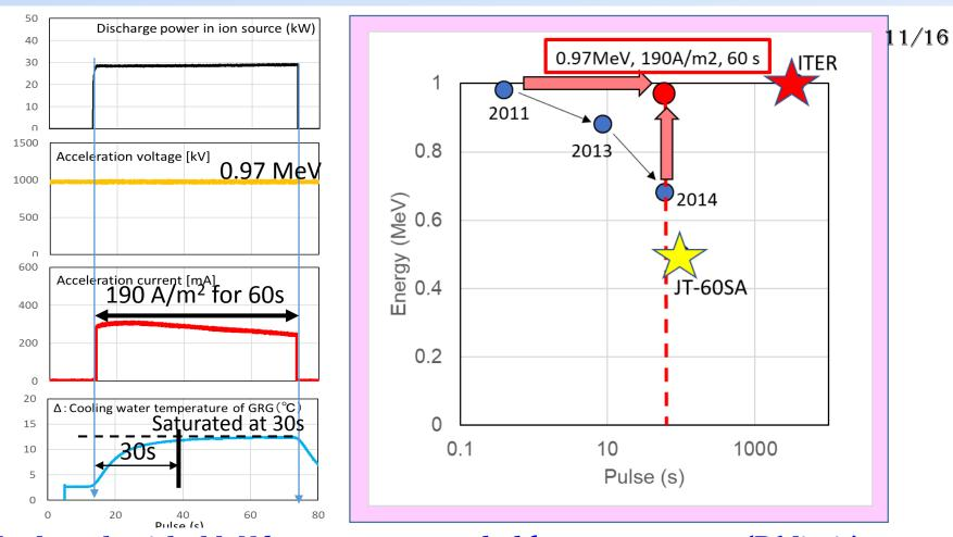
Pulse length with 1MeV beam was extended from < 1 s to 60 s (PS limit).
