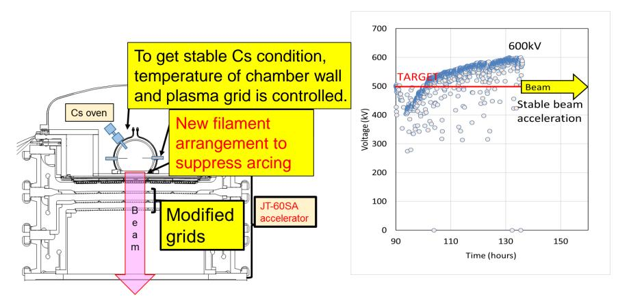
After conditioning of 600 kV with the margin of 20%, the beam was stably operated at 500keV. Now, the beam current is increasing to the target value.
