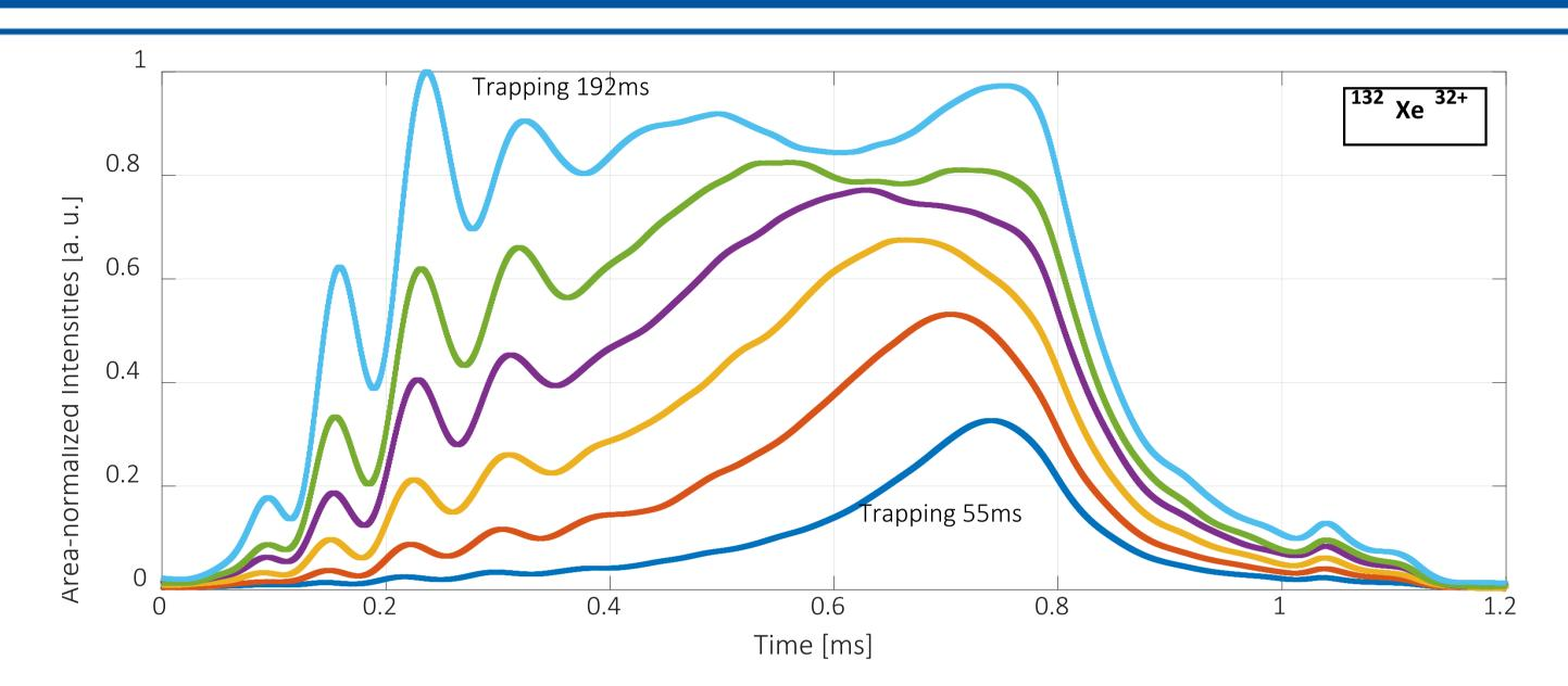
After having commissioned the Slow Extraction, several operational parameters of the REXEBIS still might be adjusted during experimental runs. The trapping time may for instance be accustomed in the case of a change of radioactive isotope to study.
