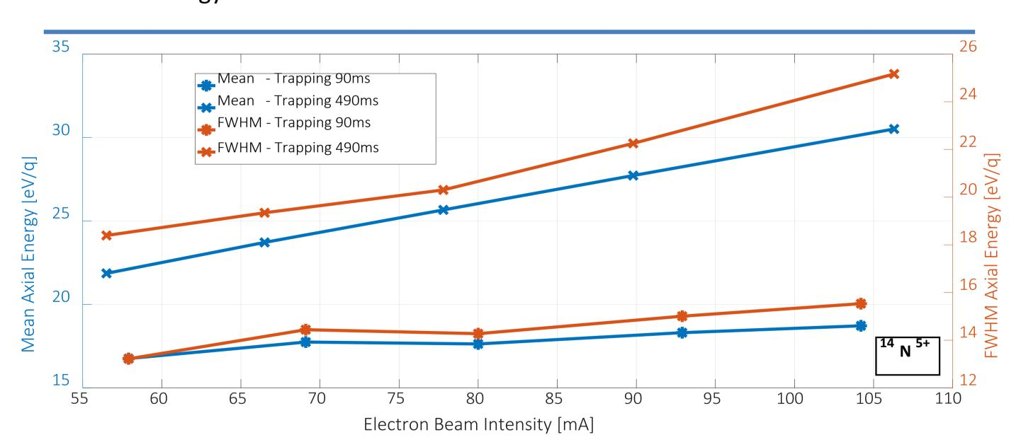
By fitting the mean axial energy as a linear function of the electron beam intensity, one obtains a ratio of 4.50 between the slopes at 490ms trapping time and 90ms. The compensation factor was measured to increase by 4.45 between 490ms trapping time and 90 ms, which can be correlated with the change in proportionality coefficients between the two linear fit functions.
