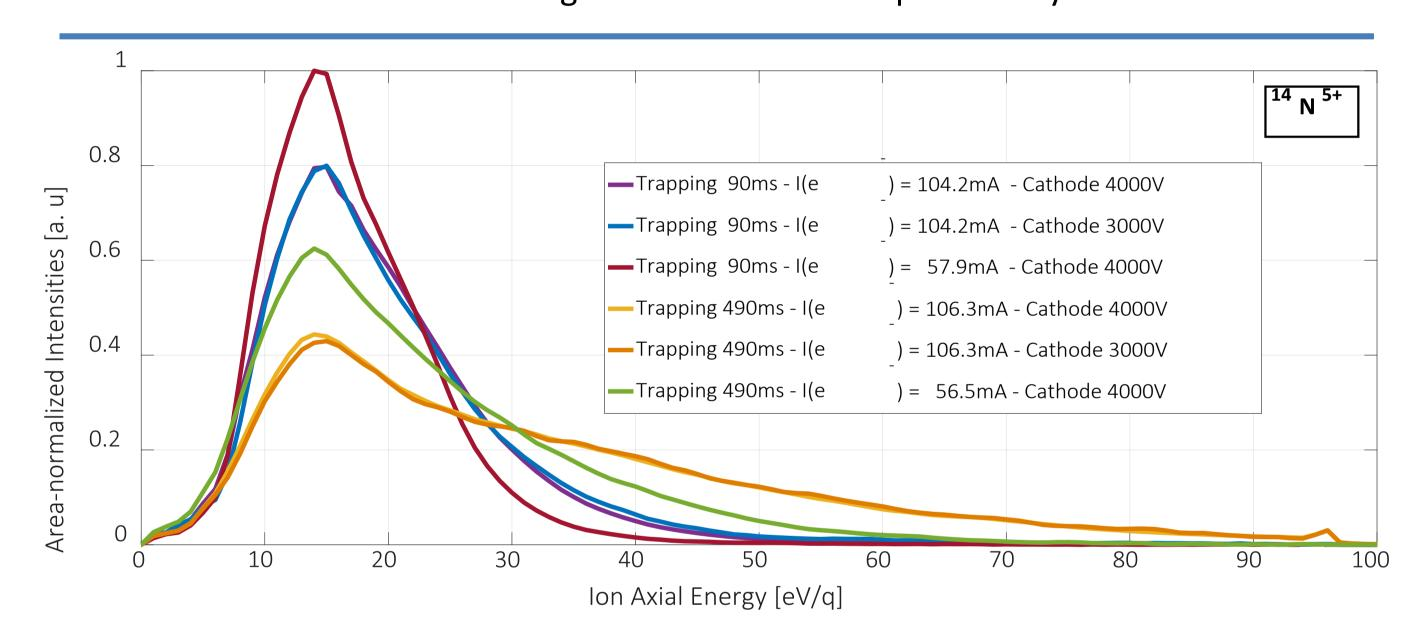
The variations of the electron beam energy within the typical range of values operated during operation, from 3keV to 4keV, were not measured to have a significant influence on the ion pulse shape. However, the trapping time and the intensity of the electron beam play a role on the ion axial energy distribution.
