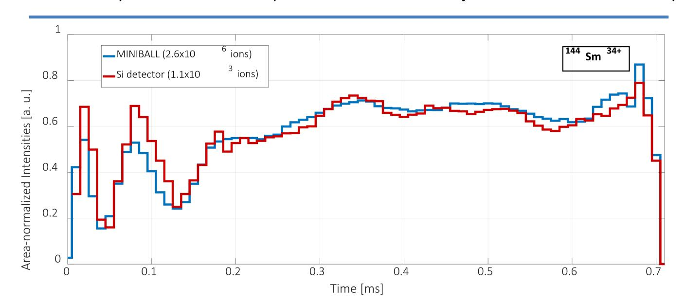
The time structure displayed, acquired with a Silicon detector and the MINIBALL spectrometer, is directly obtained from the application of Equation (1), without refinement nor fitting of the barrier voltage function. The ripples in the beginning of the ion pulse distribution are the consequences of potential differences between the drift tubes.
