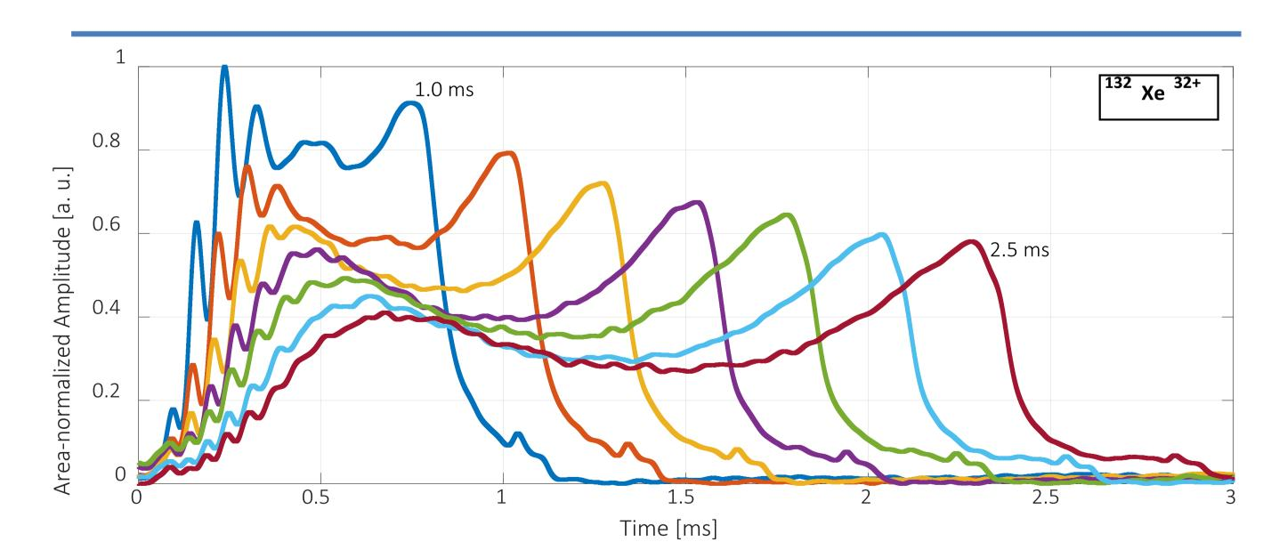
The possibility to adapt the ion pulse to a desired length is also demonstrated, notably if the prospects are to increase the Radio-Frequency systems pulse length. During the experimental runs in 2016, the average power limitation of the 9-gap IH resonator (2.5 kW), constrained the RF pulse length to be 0.7ms long. In 2017, the ensemble of REX/HIE-ISOLDE RF systems were operated with a pulse length of 1.5ms.
