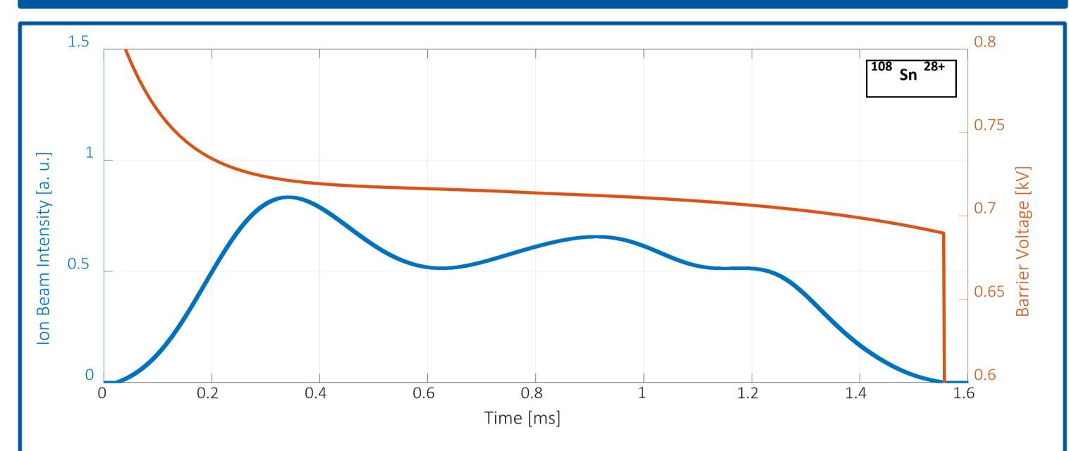
The MINIBALL spectrometer at the end of the first out of three High Energy Beam Transfer lines can provide information related to the characterization of the time-of-flight". The barrier modulation may be fit with a two-exponential function and adjusted to meet a desired shape.
