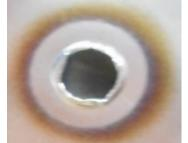
Photo of back side of tantalum collector heated by ion beam observed through a front window(top) and a collector melted by ion beam (bottom)
