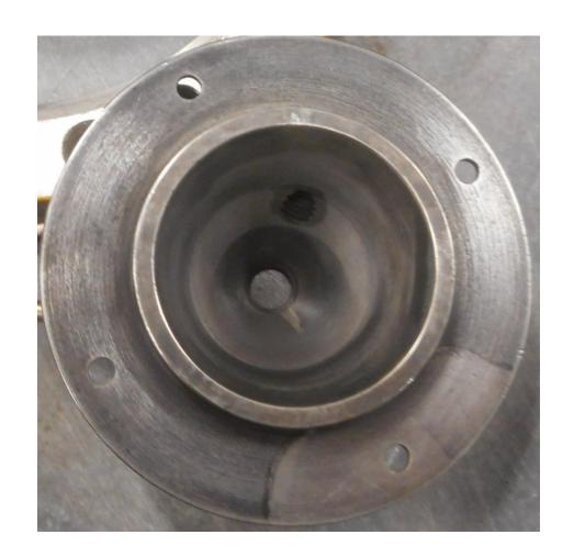
Conical collar with a dark deposition around the emission aperture
