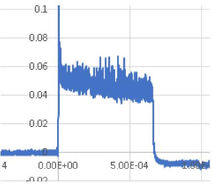
Signals of positive ion on collector Ic = 50 mA at RF power  $\sim 1.5$  kW in the plasma. The time scale is 0.5 ms/div.
