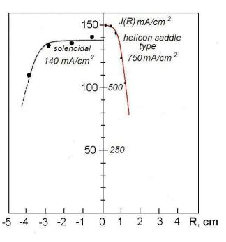
Ion flux distribution for discharge with ordinary solenoid (left) and with saddle type RF antenna (right).
