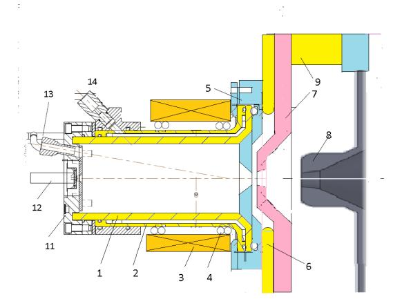
1-Gas discharge chamber (AIN), 2- cooling jacket from keep, 3- solenoid, 4- helicon antenna, 5-plasma electrode with conical collar and emission aperture, 6-extractor insulator, 7- extraction electrode, 8-grounded electrode, 9- insulator, 11- back flange, 12- gas inlet, 13- view port, 14- cooling water inlet-outlet,
