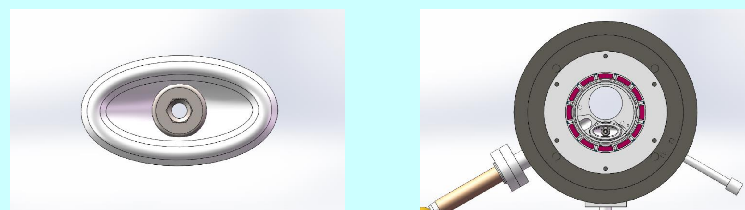
Design drawing of the hot surface ionizer and the illustration of the hot surface ionizer mounted in the ion source
