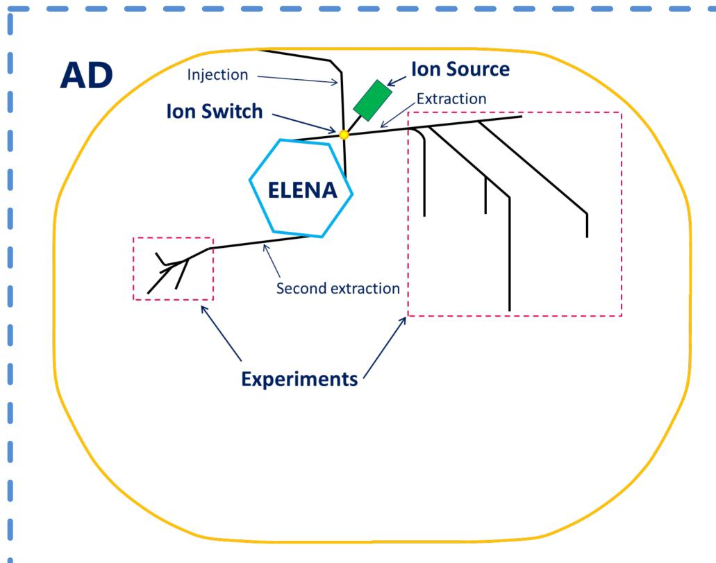
An injection line introduces the 5.3 MeV particles coming from the AD into ELENA ring. Two extraction lines are installed to guide the 100 keV antiprotons to the experiments. The H<sup>+</sup>/H<sup>-</sup> ion source is installed on the space between the injection line and the first extraction line.
