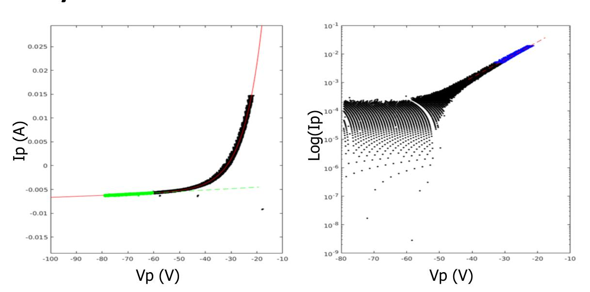
The I-V characteristic of the probe is analyzed using the following fitting formula:
