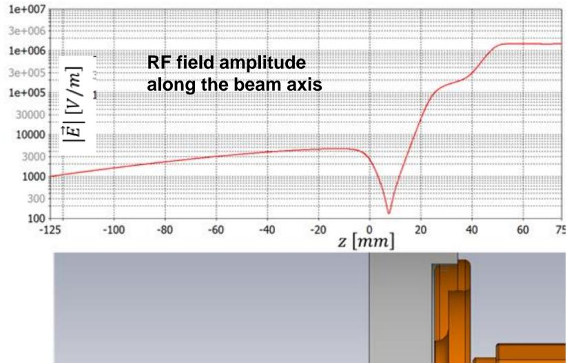
The signature of loss of the ion beam neutralization at an RFQ entrance has been observed for the first time. The initial simulations confirm that the leakage of RF field into LEBT section modifies the electron distribution and, hence, affects, the beam neutralization. It is likely that the observed phenomenon results in increased of emittance values and growth of emmitance in part responsible for modest values of the RFQ transmission. Red points – initial electrons distribution
