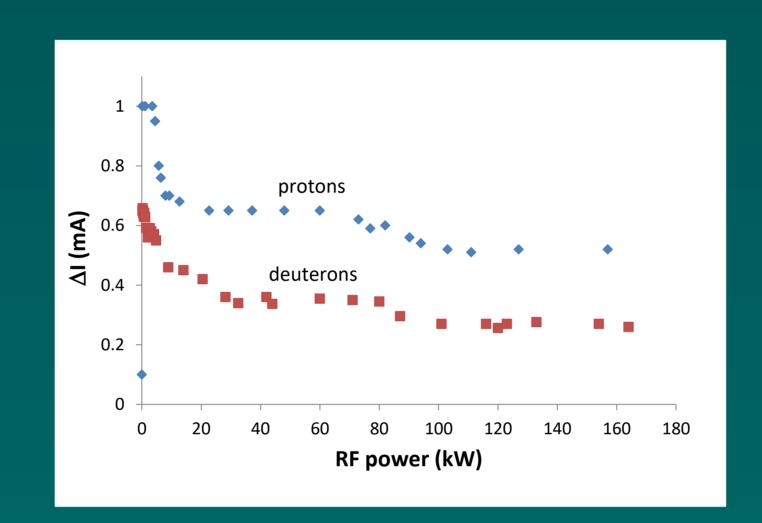
The change of beam current on the RFQ aperture with application of RF field as a function of the RF field. The effect is significantly smaller for deuterons confirming the space charge nature of the observed phenomenon.
