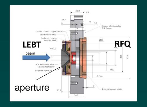
A new RFQ entrance flange has been introduced in 2014. The flange has superior cooling and RF contacts. In addition the flange has electrically insulated water cooled aperture allowing to measure the beam signal
