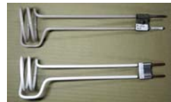
Photograph of the SNS-developed RF-antenna (upper) and a J-PARC prototype one (lower).
