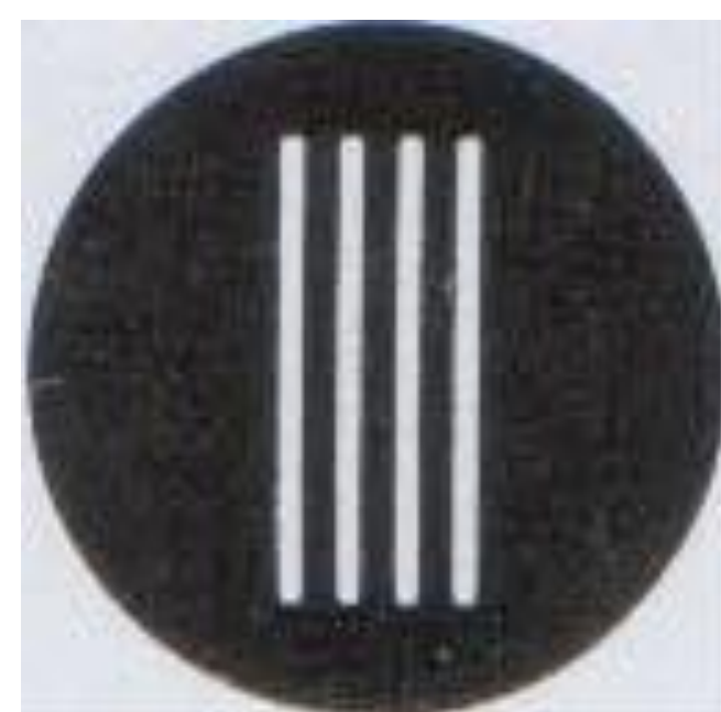
Fig. 5 Stencil mask to form irradiation pattern. The mask has 2 x 0.1 mm x 4 slits.
