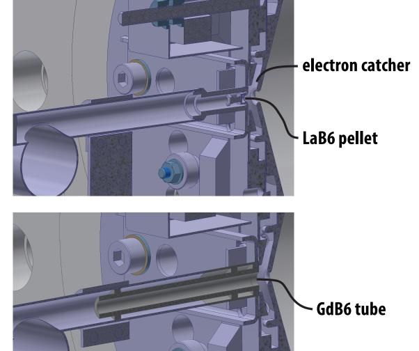
The **VADLIS** ion source aims at efficient resonance laser ionization withing a FEBIAD type ion source [3]
