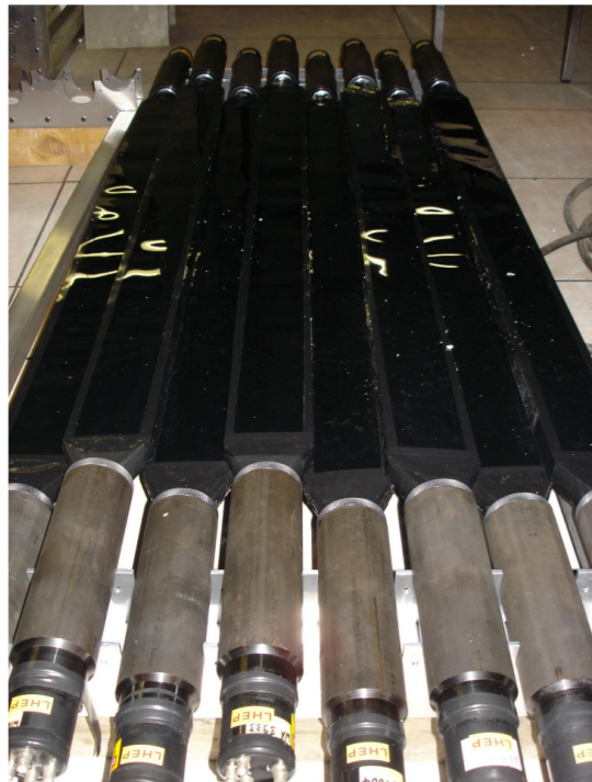
NA61/SHINE, bars with PMTs UniGe 2006
