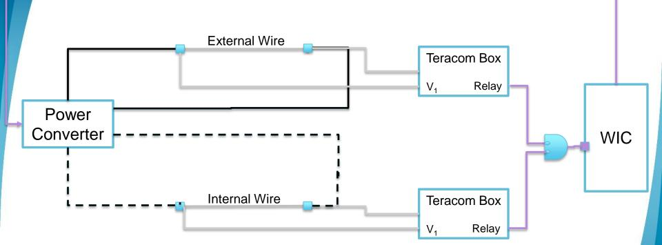
\*Diagram represents one of the sides in P5 (L or R) \*The PC can only power one wire at a time (manual switch)
