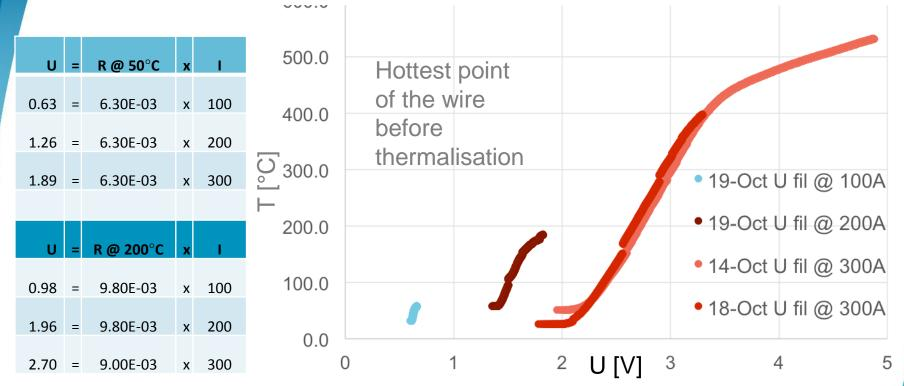
By limiting the wire tension we avoid overheating in case of loss of cooling
