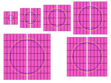
Approximately 6 layers with 220 ALPIDE sensors (fake hits rate 1000 times lower). Basically geometry of LAVD with additional layers.
