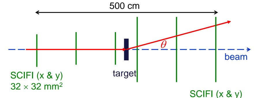
scintillating fiber detectors (X/Y projections)
