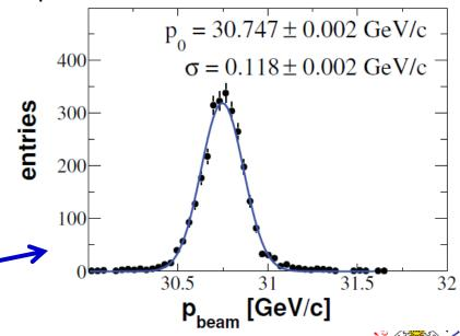
Beam momentum measurement at 30 GeV with the NA61 spectrometer at full field Almost there!
