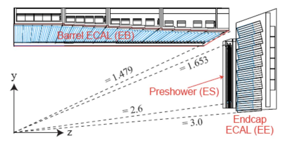
The crystal cross-section corresponds to approximately 0.0174 °— 0.0174 in  $-\eta-\phi$  or 22x22 mm<sup>2</sup> at the front face of crystal, and 26x26 mm<sup>2</sup> at the rear face. The crystal length is 230mm corresponding to 25.8 X0.
