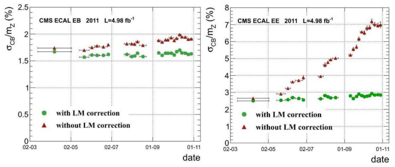
■ ECAL resolution (from Z→ee peak width) stability before and after the application of Laser Monitoring corrections (LM):
