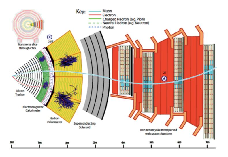
Electron identification in CMS is done measuring the shower in the crystal calorimeter and matching with the electron track. It is affected by the radiation lengths in the tracker volume, especially at  $|\eta| > 1$
