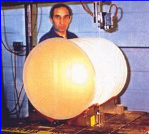
NaI:TI single crystal Ø520 mm, mass > 550 kg
