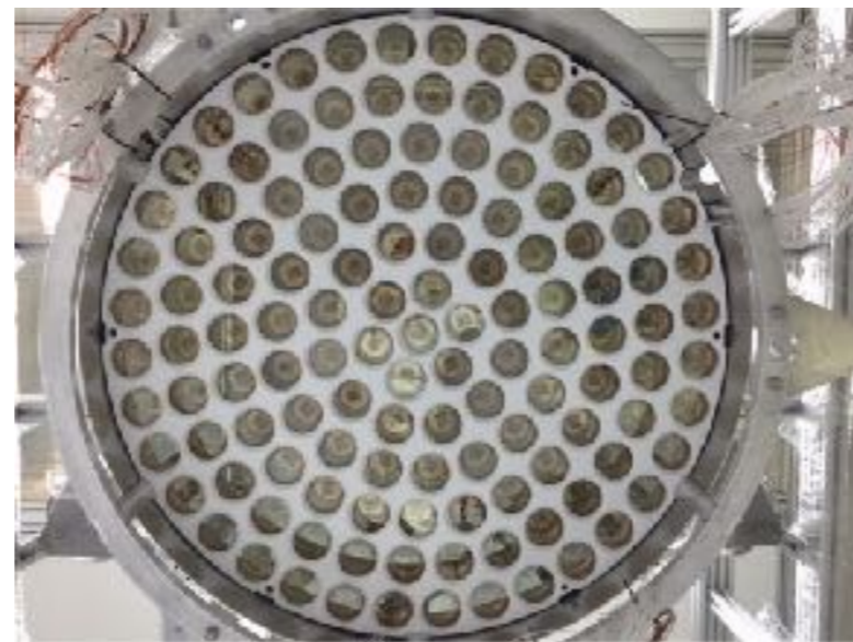
127 PMTs in the top array
