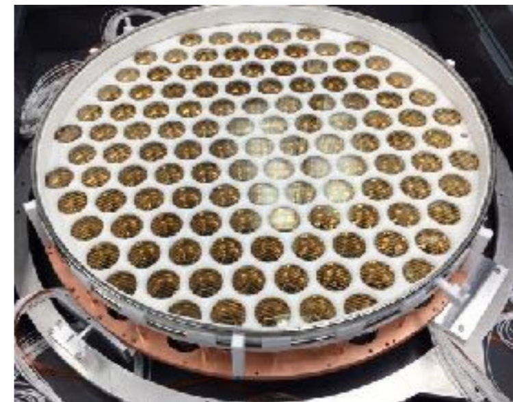
121 PMTs in the bottom array
