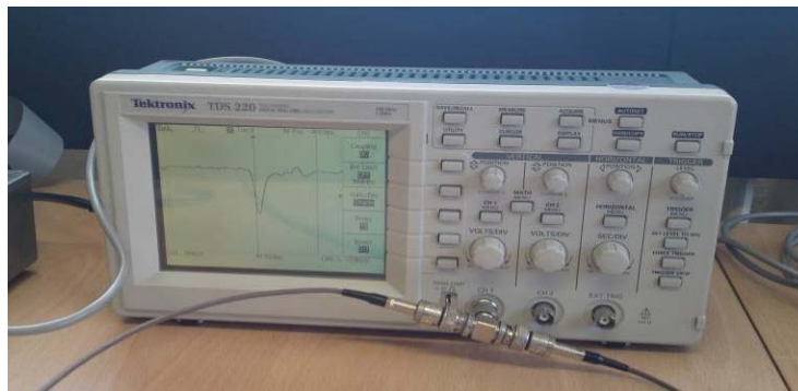
Figure 12: Example of the trigger signal on the oscilloscope.
