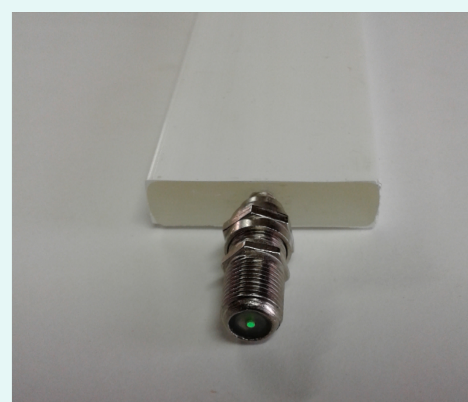
Fig. 2: MuTe employs scintillator material bars with rectangular cross-section (4cmx1cm) and 120 cm length.
