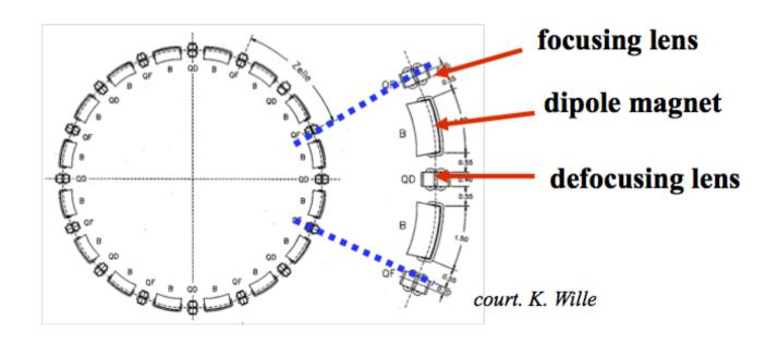
$$\begin{pmatrix} x \\ x' \end{pmatrix}_{s_1} = M \begin{pmatrix} x \\ x' \end{pmatrix}_{s_0} M_{total} = M_{QF} \cdot M_D \cdot M_{Bend} \cdot M_D \cdot M_{QD} \cdot \dots$$
