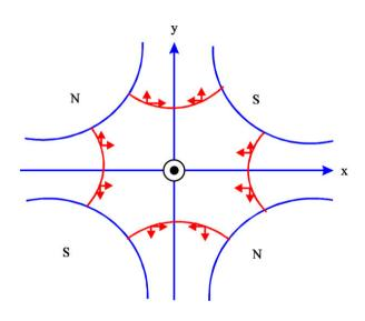
The red arrows show the direction of the force on the particle
