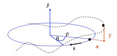
The ideal particle stays on "design" trajectory. (x=0, y=0) And:  $x,y << \rho$
