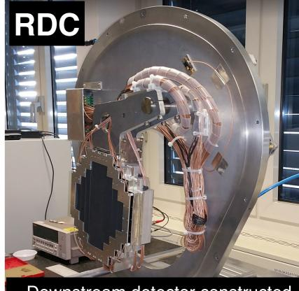
Downstream detector constructed in 2017, and performance test with muon beam finished.
