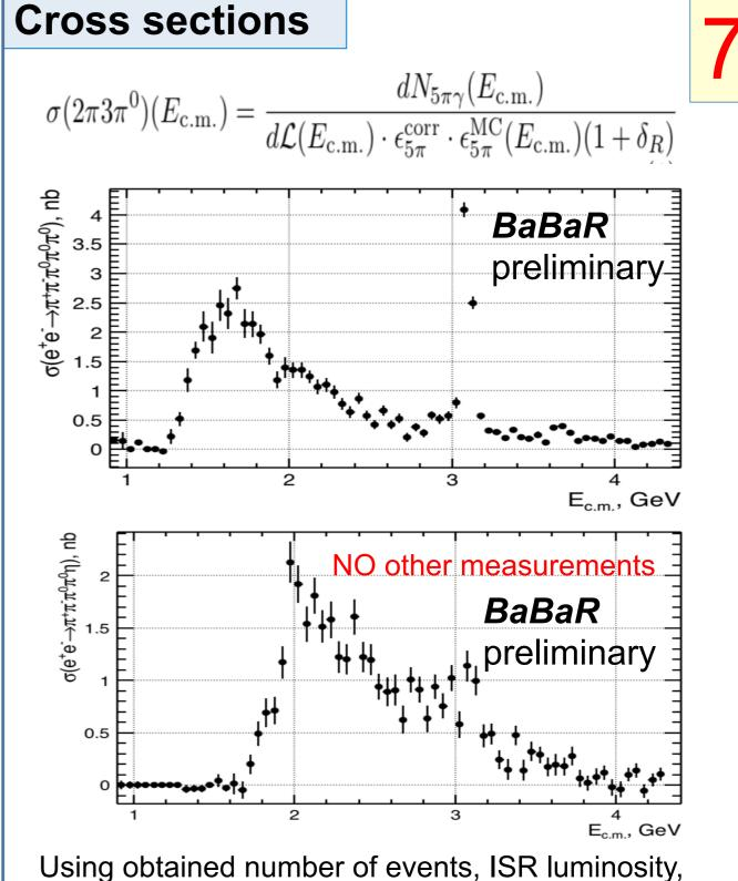
efficiency from MC, radiative correction (~1%), and correction for the data-MC efficiency difference we calculate the cross sections vs  $E_{c.m.}$  up to 4.35 GeV. Systematic uncertainties 10-13%
