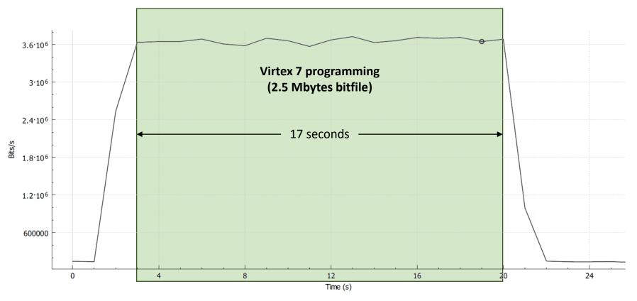
Measured using Wireshark: network transactions
