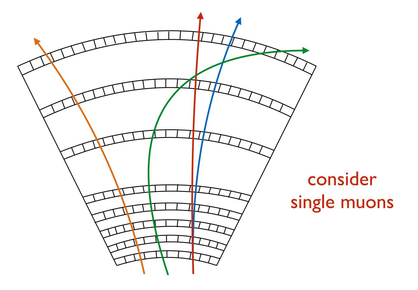
Tracks impinge the detector, leaving hits in the super-strips
