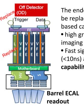
The endcap calorimeter will be replaced with a silicon-based calorimeter:
