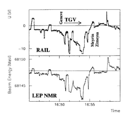
Recordings of the potential difference, U, between the rails and the Earth (top) compared with the magnetic field inside one of LEP's dipole magnets, given in units of beam energy equivalent, MeV. A strange disturbance was noticed in LEP in June 1995. A bizarre pattern in the bending magnetic field was detected for the first time thanks to new Nuclear Magnetic Resonance, NMR, probes recently installed in LEP. Small energy changes in the beam caused head scratching amongst the LEP energy team.
