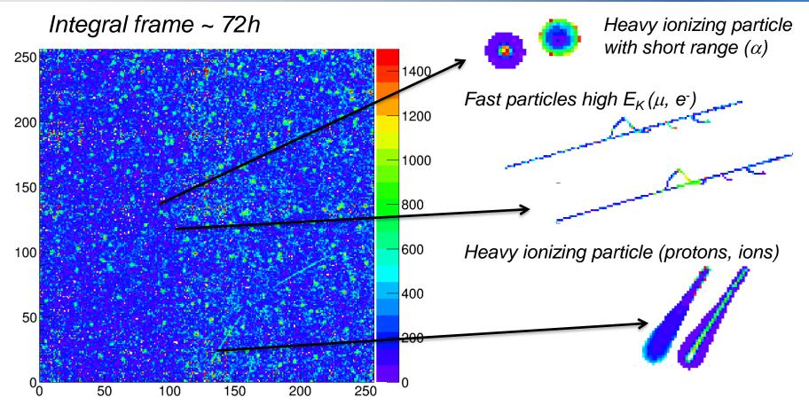
Timepix chip: matrix of 256x256 pixels Different particles present a different signature in their interaction with the pixelated semiconductor detector
