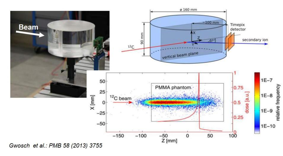
Verification in real time of the beam delivered to the patient: beam range, width and shifts in the lateral direction
