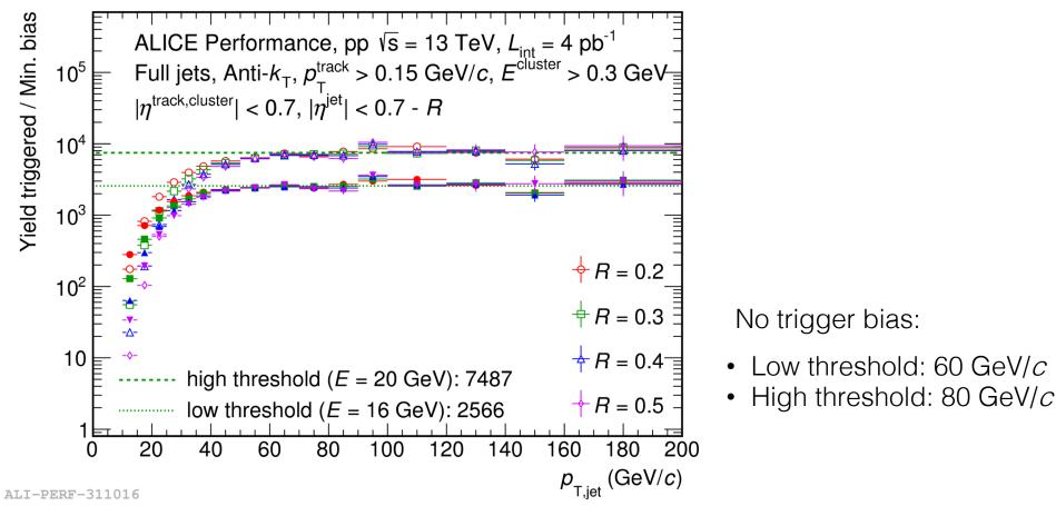
Bias free region region defines  $p_{\rm T}\mbox{-}{\rm ranges}$  where triggers contribute to substructure measurements
