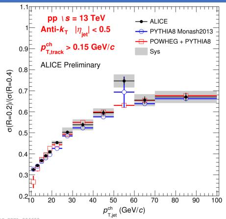
Ratios of jet cross sections with different *R* are sensitive to intra-jet broadening
