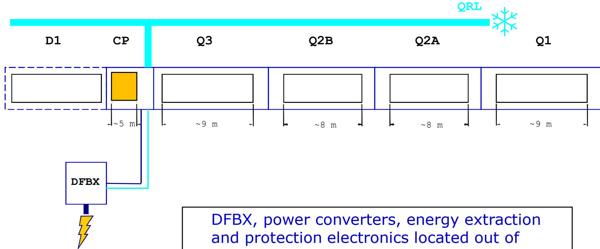
DFBX, power converters, energy extraction and protection electronics located out of tunnel, in a shielded area.
