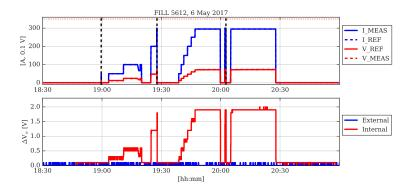
The SW interlock triggered 3 times. All triggers are fully understood. The HW interlock is set  $\Delta V_W^{thres} = 2.9$  V. We operated at  $\Delta V_W = 2$  V.
