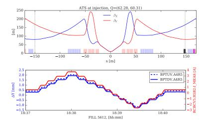
Since we could not use the 5th axis we move vertically the beam. We programmed a V bump from 2 mm at the wire.
