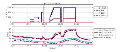
During the test we monitor constantly the temperature of the jaws. The observed  $\Delta T_{MAX} = 2$  deg as expected from workshop measurement and simulations. No special vacuum activity was observed during the full test.
