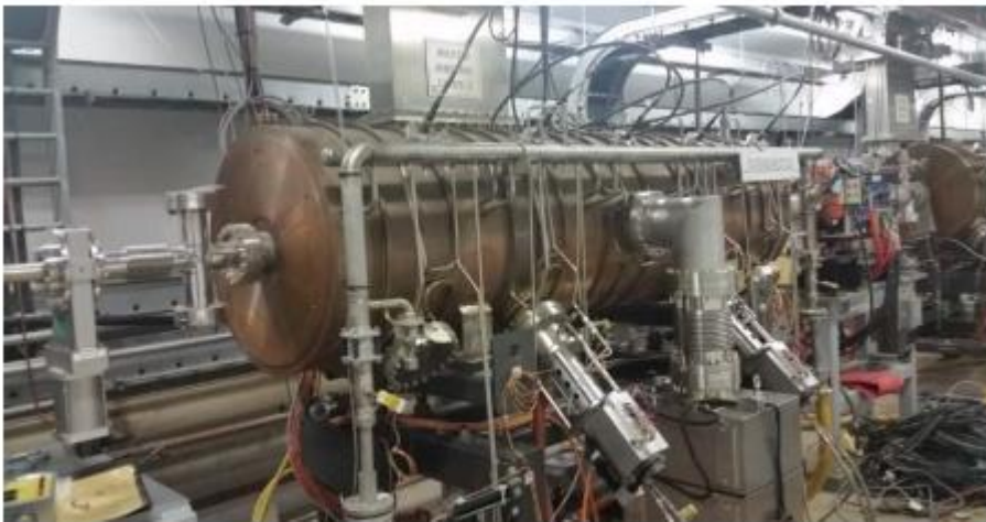
Booster has four 352-MHz, 5-cell LEP-style rf cavities.
