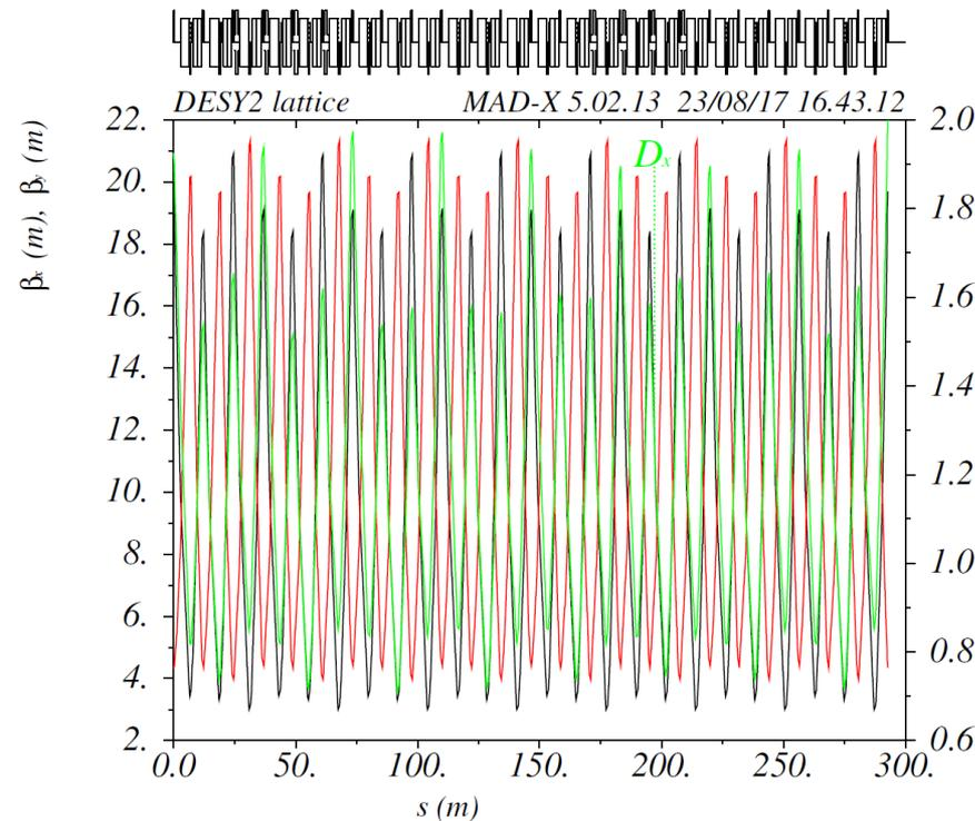
8 supercells (3 FODO cells with L=36.6m per supercell)
