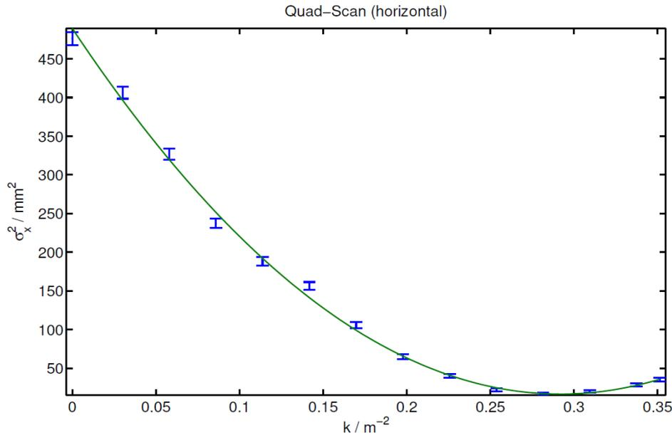
> Example of fitting of the beam size vs. the quadrupole strength for 6 GeV
