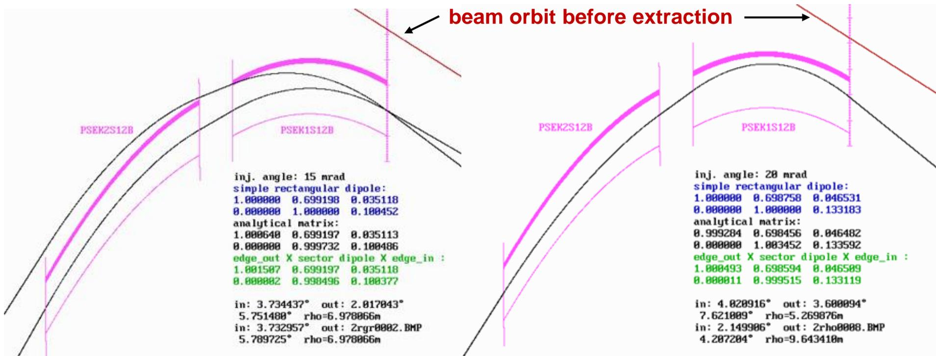
extracted beam passes very close to the septum blade where field deviates from a pure dipole – to first order this corresponds to a defocusing gradient
