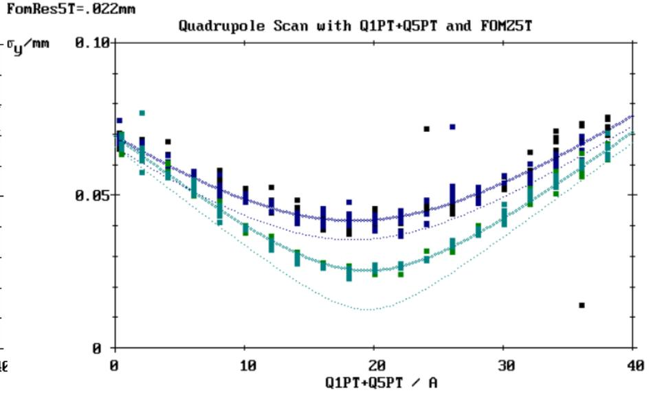
dots are experimental results, thick line predicted dependance, thin line – true beam size
