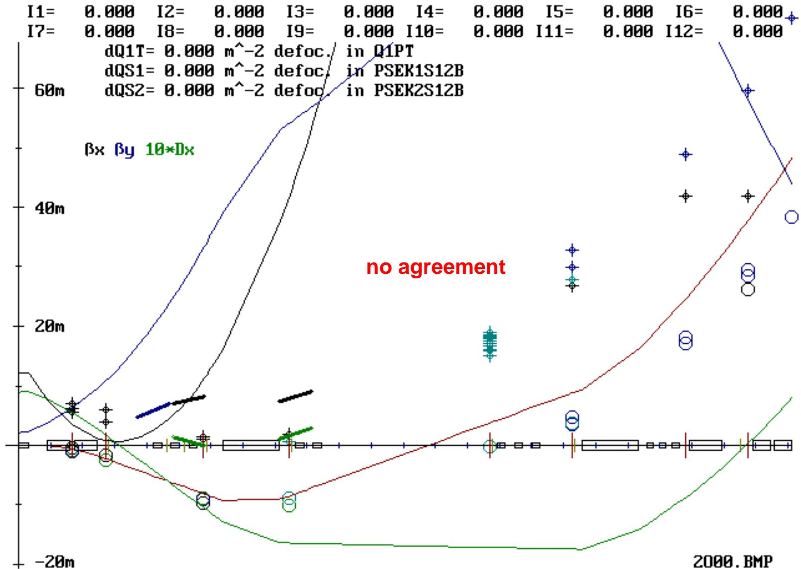
due to entrance angle of extracted beam and displaced septa the actual orbit differs significantly from the design orbit:
