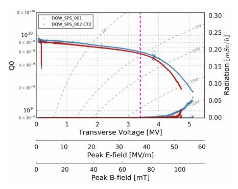
Both cavities exceeded the 3.4 MV requirement. The heat load is instead higher than the initial goal. This triggered discussion on numbers to choose as a baseline. In light of the fact that the Q factor was a very rough and old estimation (before any actual data), it has been decided that the threshold of dynamic load per cavity is formally set to 5 W at the nominal voltage of 3.4 MV. Carlo said such a value is already included in the last MME official heat loads estimations.
